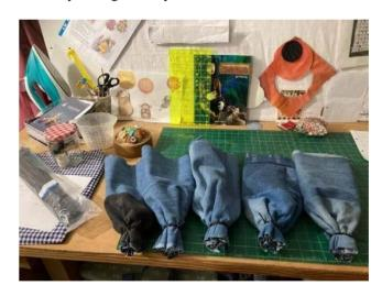
As you can see, the final product is rather crude. The sewing machines couldn't cope so we used cable ties to close up the bottoms to make sure the ball of the clapper was fully covered and nothing slipped. The bags are pushed up over the clapper as if putting a bottle of wine in a bottle bag and another cable tie or two is put round the top above the clapper.
